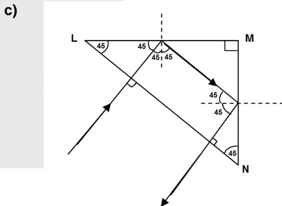
Light enters the prism from face LN perpendicularly and hence does not refract. It then hits the surface LM at  $45^\circ$  which results in total internal reflection as the angle of incidence is greater than the critical angle. It then hits MN and also undergoes total internal reflection there because its angle of incidence is  $45^\circ$ . Hence it escapes from the surface LN.
