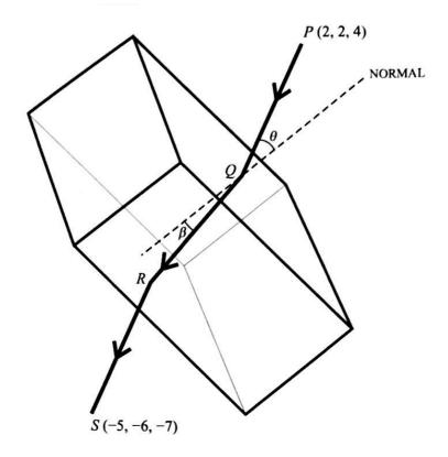
A ray of light passes from air into a material made into a rectangular prism. The ray of light is sent
